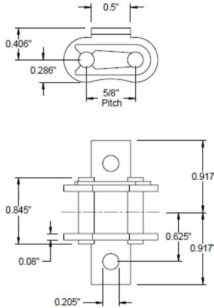
**Figure 6: ANSI #50 Chain Attachment Piece**
