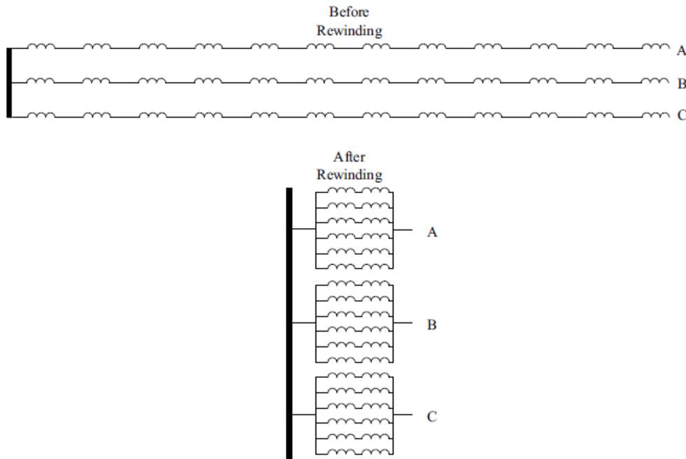
Figure 1: Rewiring the Generator
