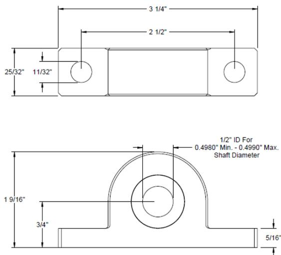
**Figure 5: Mounted PTFE Sleeve Bearing**
